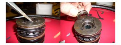
2. Insert the BMX-4 tool into the 4 holes on the 800-3744 - Clutch Axle JGS and attach the adjustable spanner to the BMX-4 tool.
