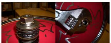
3. Untighten the Clutch assy using the BMX-4 tool and the adjustable spanner. Turn Anti clockwise to untighten, so the tool does not come out while unscrewing I recommend placing a screw threw the flywheel assy to keep the tool in place.
