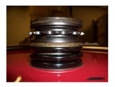
1. Using a flat Screwdriver and a rubber hammer to gently tap the locking nut Anti-clockwise until this becomes loose enough to unscrew by hand.
